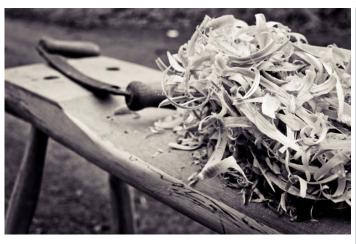
very twisted, and also a very hard wood when it is dry. But the holly was very hard to work – very dense, very wet, and in the end the mushrooms split too easily after working, early on in the drying process. I will probably leave the remaining holly poles to dry a bit before working them.
