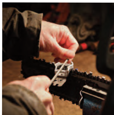
Filing a chain with a Husqvarna roller guide.
