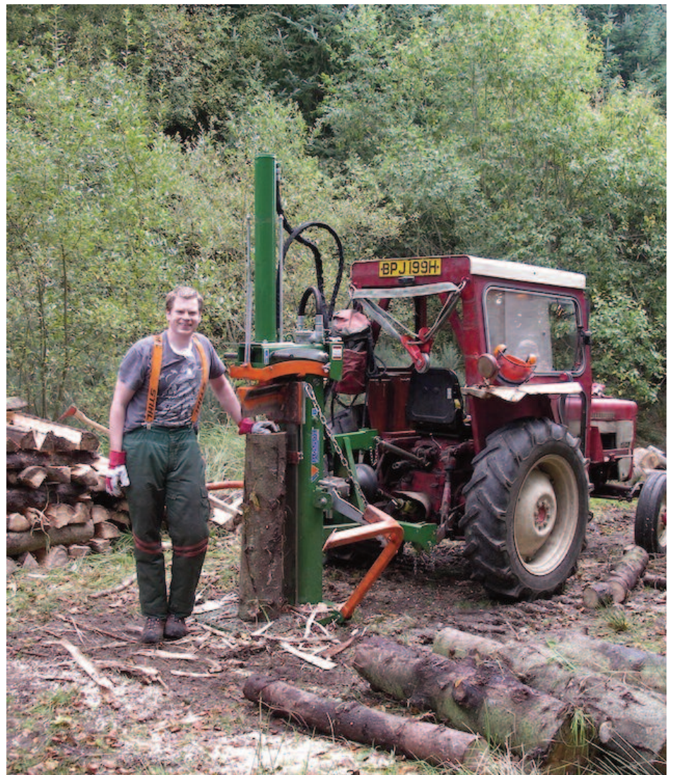
Below: Cameron's son-in-law Jonathan, with the Posch 20T log splitter, which runs off the tractor PTO.
