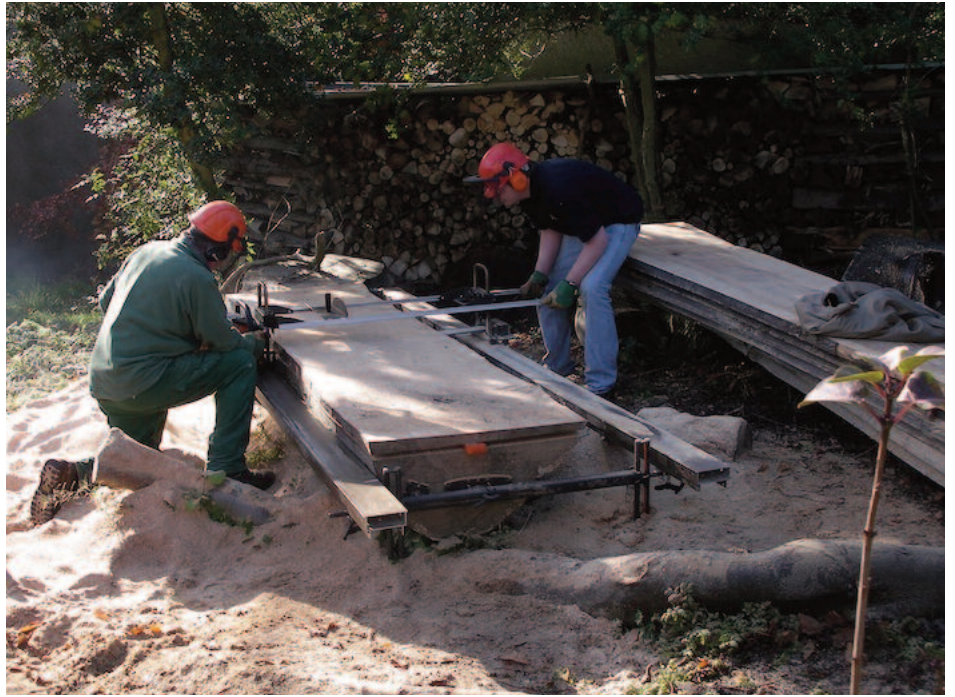
Above: Pro system, with an MS 650 doing the cutting, on a beech trunk.
