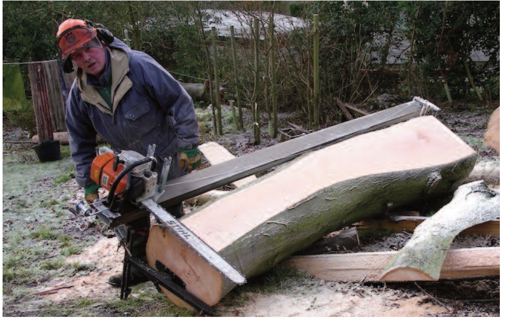
Big Mill planking system in operation, with Cameron at the saw.
